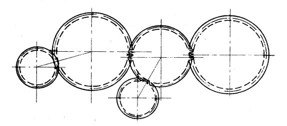
Fig. 9 Timing gear meshing signs
