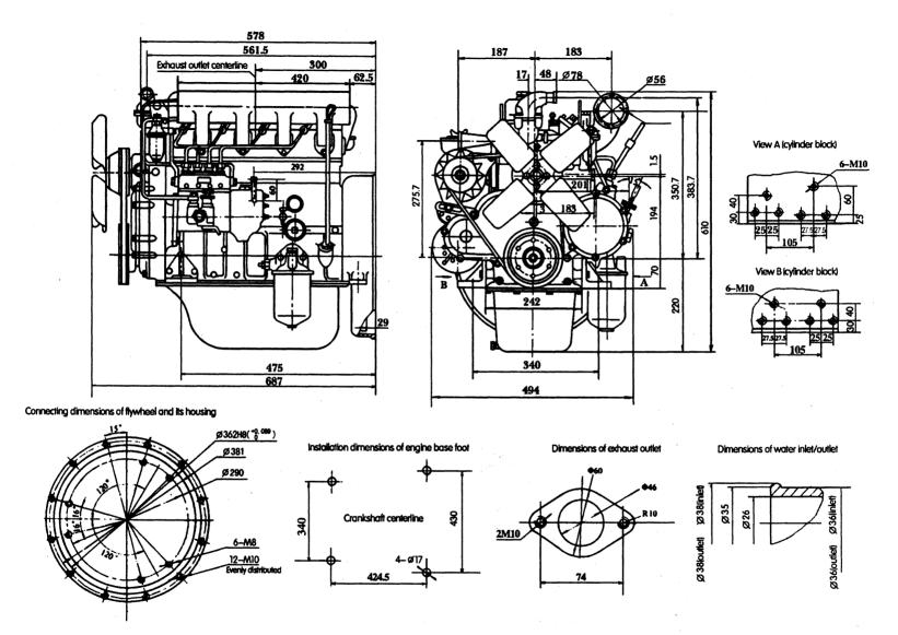
I. Configuration and Installation Dimensions of Model Y480 Diesl Engine
