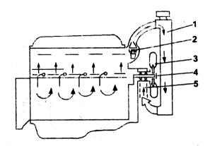
Fig. 12 Cooling system 1. Radiator 2. Thermostat 3. Cooling fan 4. Water pump 5. Inlet water pump
