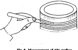
Fig. 8 Measurement of side surface gap of piston ring
