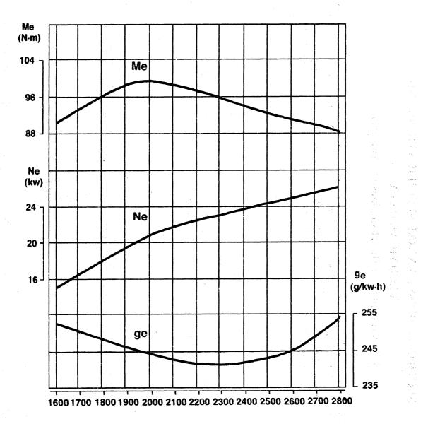
II Performance Curves of Model YD480 Diesel Enging
