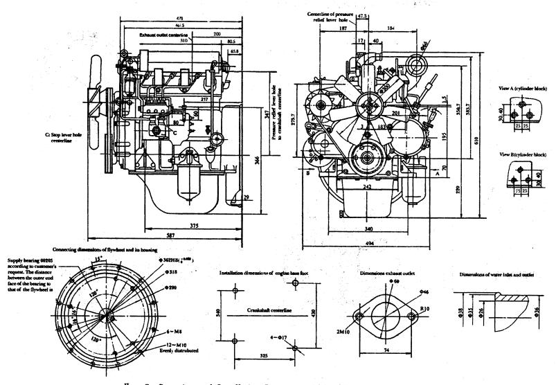
${\rm I\!I}$  . Configuration and Installation Dimensions of Model Y380 Diesl Engine
